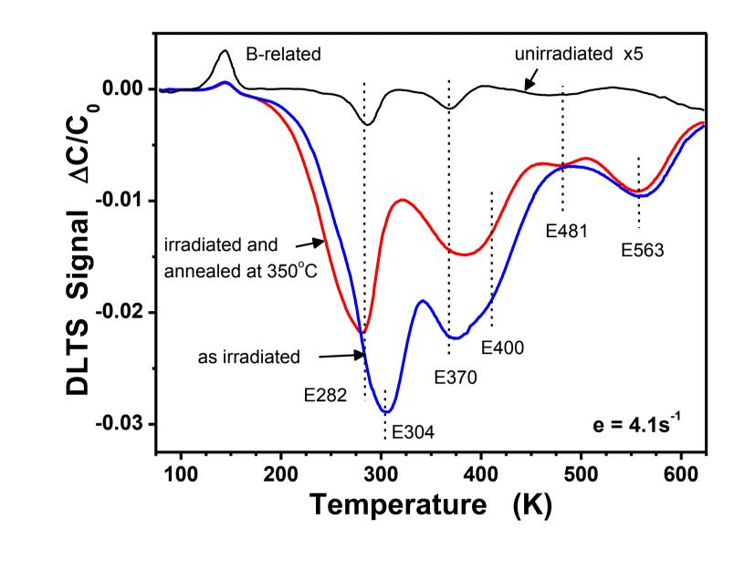
**Carrier Removal by Neutron Irradiation**
