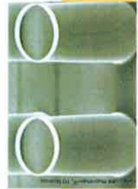
GaAs-AlGaAs-Bragg reflector of VCSELs. Deep etching of quartz
