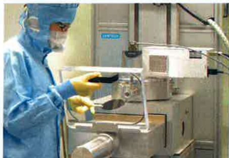
Atomic Layer Deposition system SI ALD LL with true remote plasma source and loadlock
