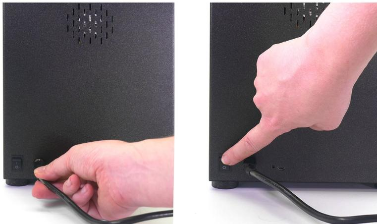
*Connecting the power supply unit and turning on the machine*
