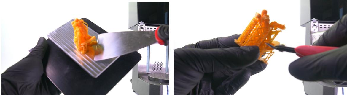
*Use a metal spatula to remove the printed object from the printing platform. You can also consider removing the supports at this point.*
