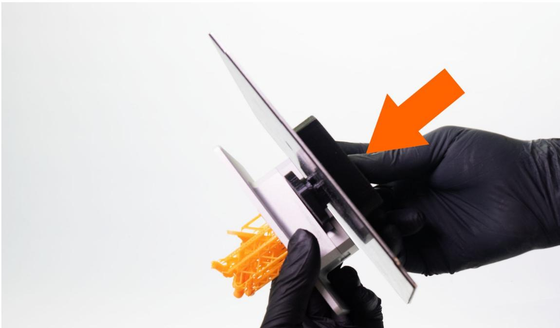
Now place the **lid on top of the liquid container** so the print is **submerged** in isopropyl alcohol. This is the recommended procedure, because both the platform and the object are washed.
