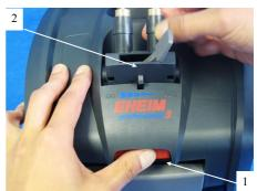
Insert the funnel into the right-hand side fill hole (1).
