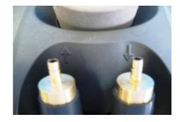
Push the tubing firmly to the inlet and outlet nozzles.
