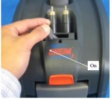
Unclip the four grey plastic catches from each side of the ECP. The catches are released by pulling the grey lever outward from the bottom.
