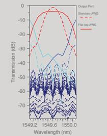
BeamPROP simulation of an at-top AWG. The taper on the input port was designed to produce the at-top response shown. The standard AWG output is also shown as reference.
