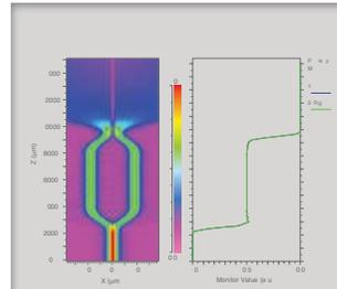
BeamPROP simulation of a Mach-Zehnder modulator operating completely out of phase. The power in each arm is shown on the right.
