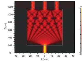
BeamPROP simulation of a  $1 \times 3$  MMI device. The length of the MMI was optimized so that the three output waveguides contained equal power.
