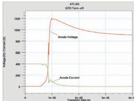
The calculated anode current and anode voltage during turn-off.
