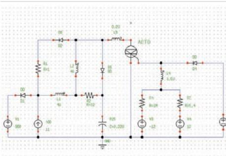
This circuit is used to investigate GTO turn-off. The GTO is a physically-based device whereas compact analytical models are used for the four diodes.
