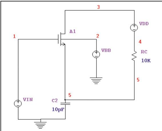
This charge pump circuit provides a standard test of the ability of a device model to conserve charge. The circuit is simulated using MixedMode, with transistor A1 simulated as a physically-based device.
