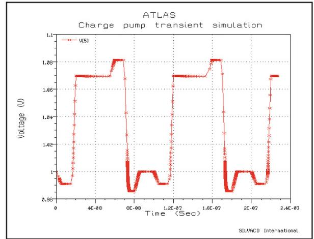
The voltage waveform on the source of the MOS transistor (node 5) has a steady DC level. This demonstrates that charge is conserved.
