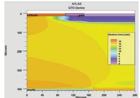
The carrier concentration within the physically-based device can be examined at any time during the circuit transient.
