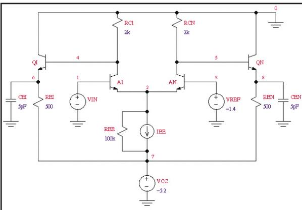
This circuit is an ECL inverter. Transistors AI and AN are simulated as physically-based devices, and transistors QI and QN are simulated using compact analytical models. The calculated base and collector waveforms of the devices are shown in the adjacent figure.
