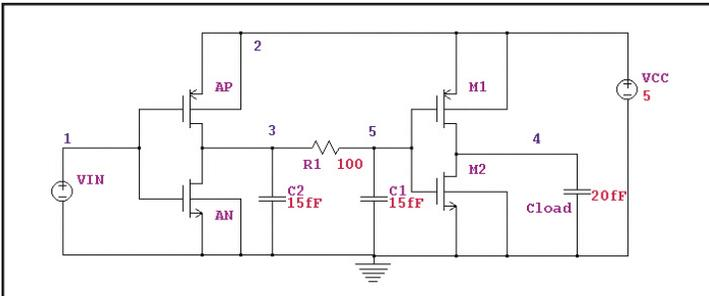
The circuit above shows a CMOS inverter loaded by interconnect parasitics and another inverter. Transistors AP and AN are simulated using physically-based devices and transistors M1 and M2 are simulated using compact analytical models.
