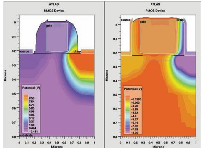
Conditions inside the two physically-based devices. The conditions inside multiple physically-based devices can be displayed simultaneously. Animation showing the evolution of internal conditions is easily generated.
